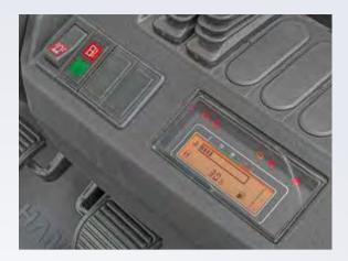
Newly developed LCD meters have more complete functions and more stable performance. Important information including running status of the entire truck and failure of the engine (electronically controlled engine) can be displayed completely, so that the operator can understand status of the truck in a visualized manner, for easy maintenance.
