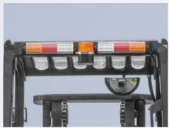
LED lights are applied for entire truck. It saves power and energy, with significantly increased performance and service life of lights.
