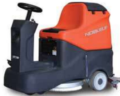
NR530 21" Brush with 30" Squeegee 18.5 Gallon Capacity Tank Electric Ride-On Scrubber
