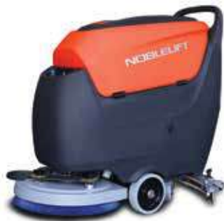
NB530 21" Brush with 30" Squeegee 13.2 Gallon Capacity Tank Electric Walk-Behind Scrubber
