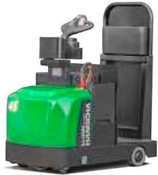
Lithium-ion Stand-Up Tow Tractor 10,000lbs 24V/404Ah
