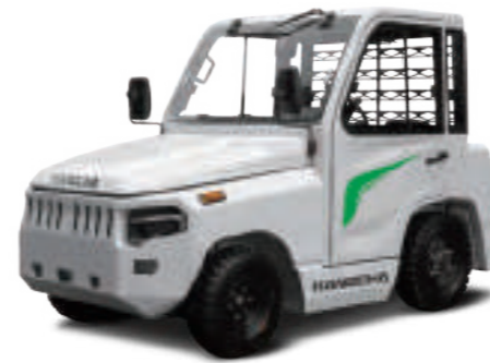
Lithium-ion Heavy Duty Tow Tractor 44,000-70,000lbs 80V/404Ah, 80V/542Ah, 80V/808Ah
