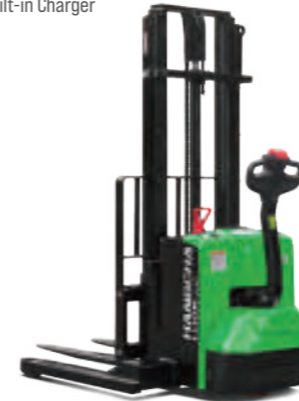
A Series Lithium-ion Industrial Walkie Counterbalanced Stacker 2,000-4,000lb Load Capacity 24V/404Ah
