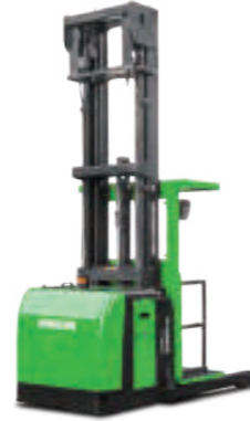
A Series Electric Lithium-ion Four-Wheel High Level Order Picker 3,000lb Load Capacity 36V/813Ah
