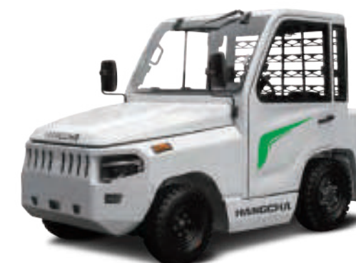
X Series Electric Lithium-ion Heavy Duty Tow Tractor 44,000-70,000lb Towing Capacity
