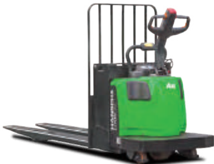
A Series Lithium-ion End Control Rider Pallet Jack 6,000-8,000lb Load Capacity
