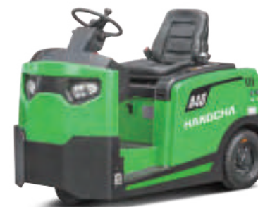
A Series Electric Lithium-ion Tow Tractor 4,500-13,500lb Towing Capacity
