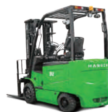
X Series Electric Lithium-ion Cushion Tire Forklift 3,000-6,500lb Load Capacity
