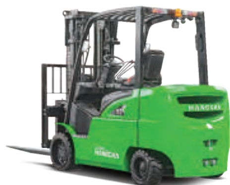
X Series Electric Lithium-ion Cushion Tire Forklift 8,000-12,000lb Loading Capacity
