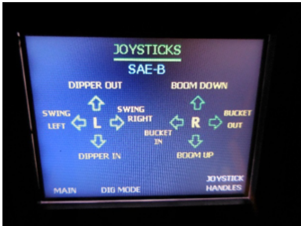
Figure C-5b: Joystick movement is SAE Dig Mode
