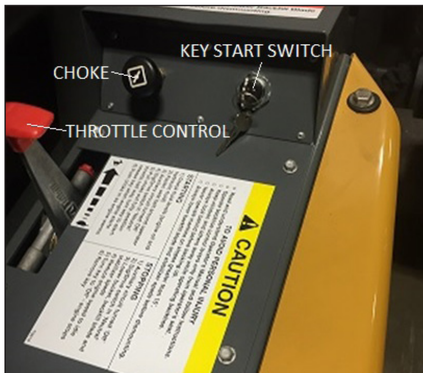
Figure C-6: Side Control Panel: Key start switch, choke (on gas model) and throttle control
