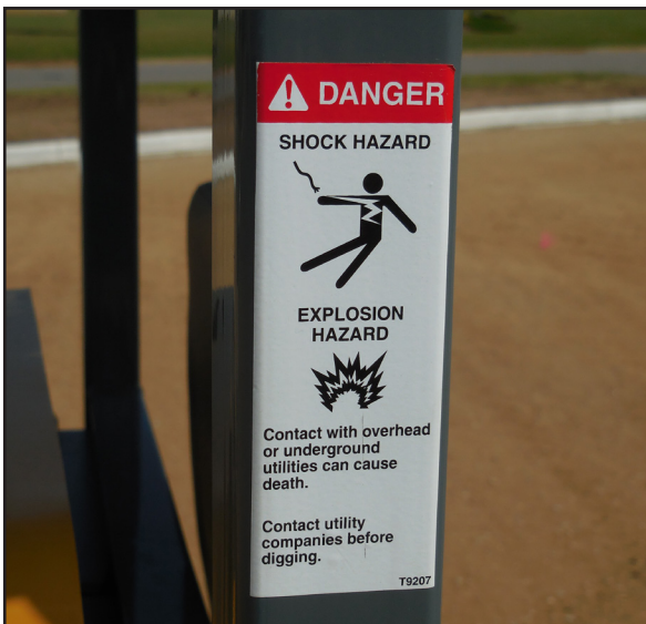
Electrical shock hazard, located on multiple locations boom, and both sides of ropes T9027 (x3)
