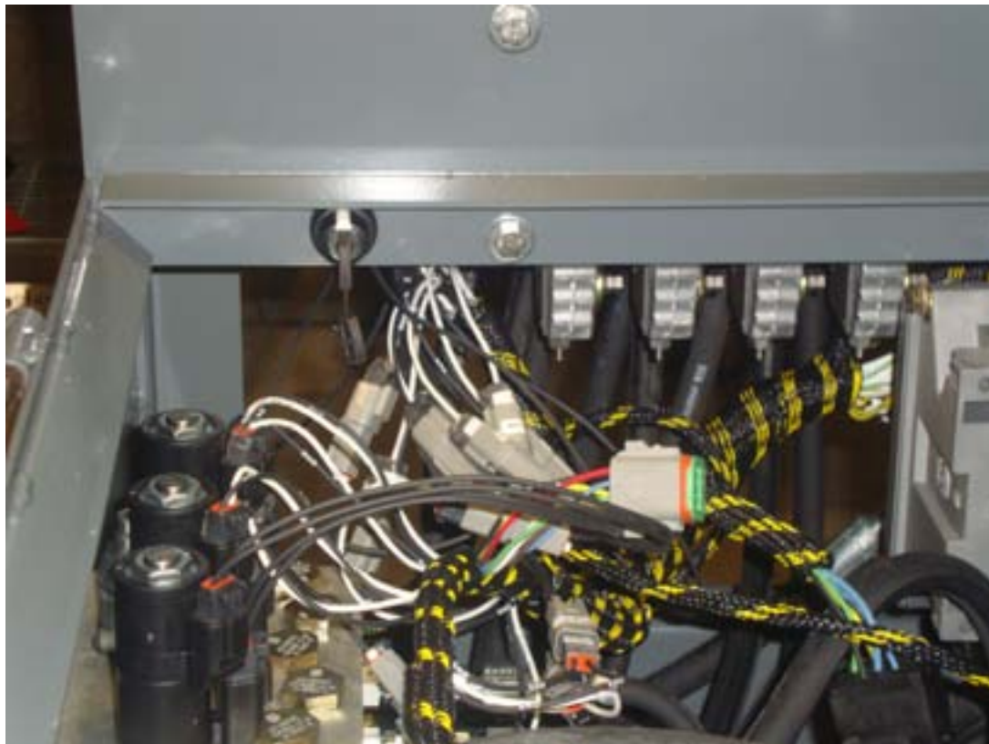
Figure C-3: Speed control, located under the seat, is a 3-position keyed switch shown in middle position (shipped in this configuration.) Turn to the left for low speed and to the right for high speed.
