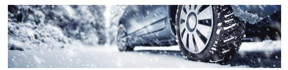
According to Consumer Reports' testing, a tire's tread depth is essential to disperse rainwater, slush, and snow. As tires wear, this ability to hold the road confidently diminishes.
