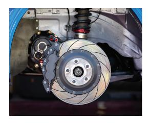
**Vibrations:** If your steering wheel shakes when you brake, it could mean your rotors are warped.
