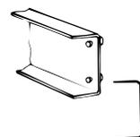
Higher capacity left-to-right support for bulk storage decking. 3" x 7/8"; 14 gauge. Channel beams cannot be located directly at floor level due to their longer face. For a beam level directly at floor level, use angle beams with support ties.
