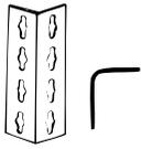
Standard duty upright post. Supplied with starter units. Use on freestanding units and row ends of units or runs of units. 1.57" x 1.57"; 14 gauge. Punched on 1-1/2" centers
