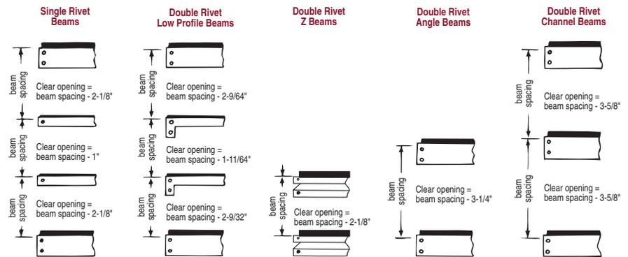
Vertical clearance calculated using 5/8" thick decking material
