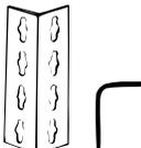
Designed for maximum load capacity and stability. 1-7/8" x 1-7/8"; 14 gauge. Punched on 1-1/2" centers.
