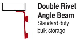
**Double Rivet Angle Beam**
