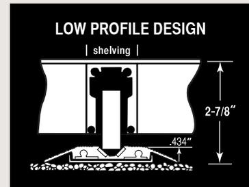
Steel wheels roll on steel strips encased in aluminum tracks.
