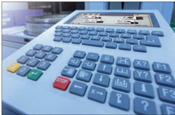
Hänel microprocessor control system MP 12 N-S with touchscreen technology and integrated storage management
