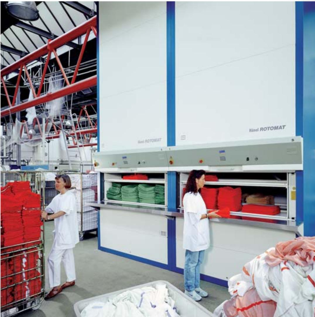
This Rotomat® system has one access point at the front and one at the back. The ironed laundry is stowed away at the back and taken out as needed from the front.
