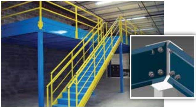
COLD-FORMED C-CHANNEL The most efficient and economical system for short to medium column spans.
