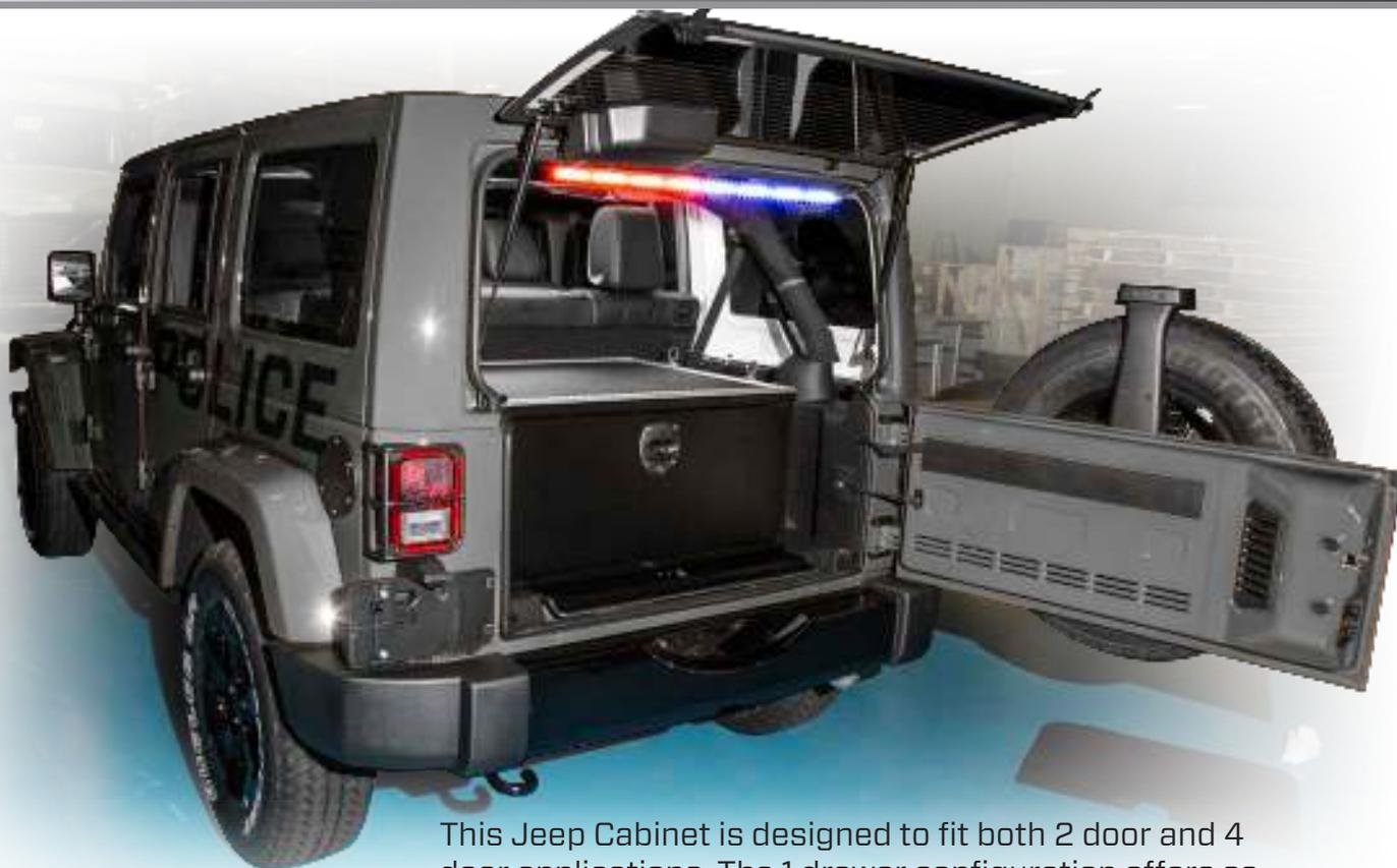
This Jeep Cabinet is designed to fit both 2 door and 4 door applications. The 1 drawer configuration offers secure storage with additional storage on top.
