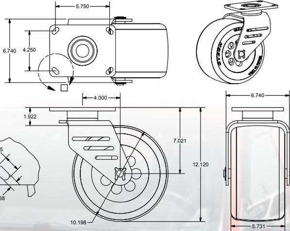
The 10" Bad Ass Caster allows for easy maneuverability over all terrains. Designed to roll like a pneumatic tire while maintaining the load capacities of a caster. These carts are designed for extreme conditions for a caster application and outfitted with 2 swivels with brakes and 2 fixed casters on all standard carts.
