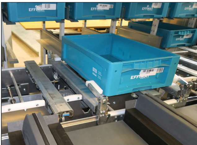
Intelligent Box Mover Technology allows boxes to be moved horizontal
