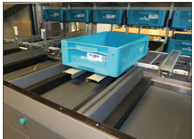
The extractor presents up to five different boxes in each working cycle
