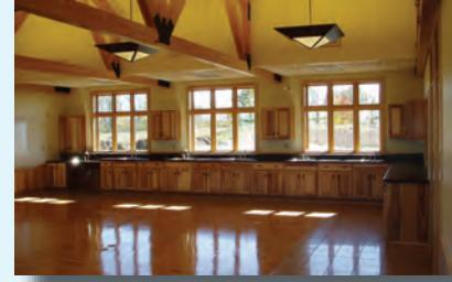
Cool daylighting involves configuring the building design to harvest and take advantage of natural light, without allowing direct penetration of sunlight in the spring, summer and fall, to reduce electricity usage for lighting and reduce the need for additional mechanical cooling.
