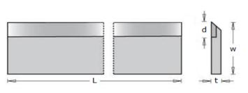
DESIGNED FOR COST-CRITICAL APPLICATIONS. CARBIDE TIP PLANER KNIVES & ECONOMY CARBIDE TIP KNIVES STILL OFFER BENEFITS OF CARBIDE, BUT COST IS CONTROLLED BY USING A THINNER CARBIDE THICKNESS (1/32") THAN CENTRIC C.T. KNIVES.
