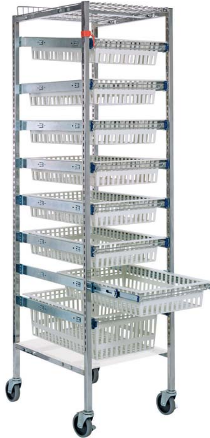
PS-S2475-8PT Starter Unit with Plastic Mesh Trays 24"D x 19-1/2"W x 75"H 7 - 4" trays with 1 Long & 2 Short-Dividers 1 - 8" tray with 1 Long & 1 Short-Divider 1 - safety stop 1 - bottom dust cover
